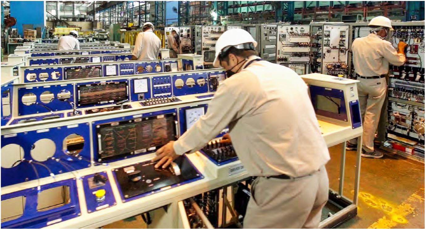
Control System Manufacturing at Switchgear Division (SCR), BHEL Bhopal for DETC (Diesel Electric Tower Car)
