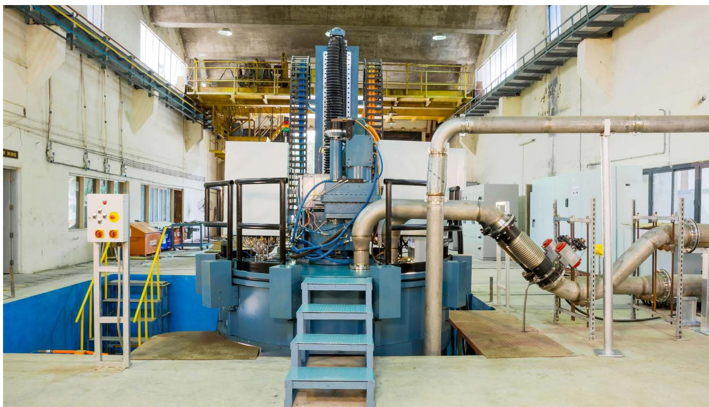
*Unique High Temperature Spin Test Rig (HTSTR) established for testing of advanced materials for AUSC mission project*
