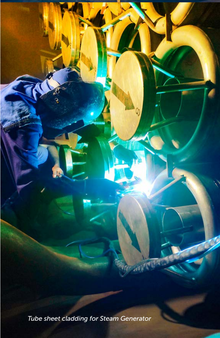
Tube to Tubesheet Welding for Nuclear Steam Generators
