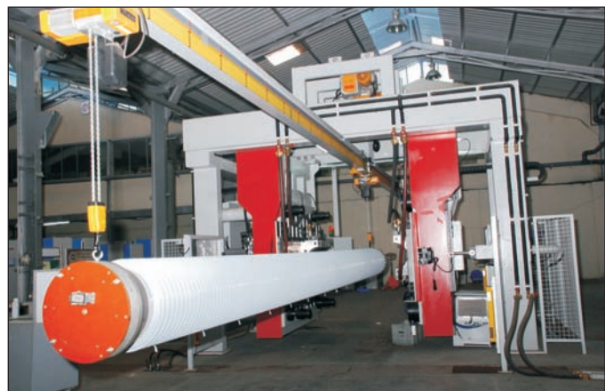
800 kV Polymer composite insulator - under manufacturing at EPD Bengaluru
