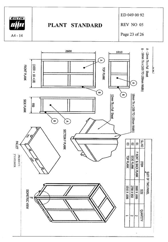
Fig - 11 : Plywood Packing for 2suit panel.
