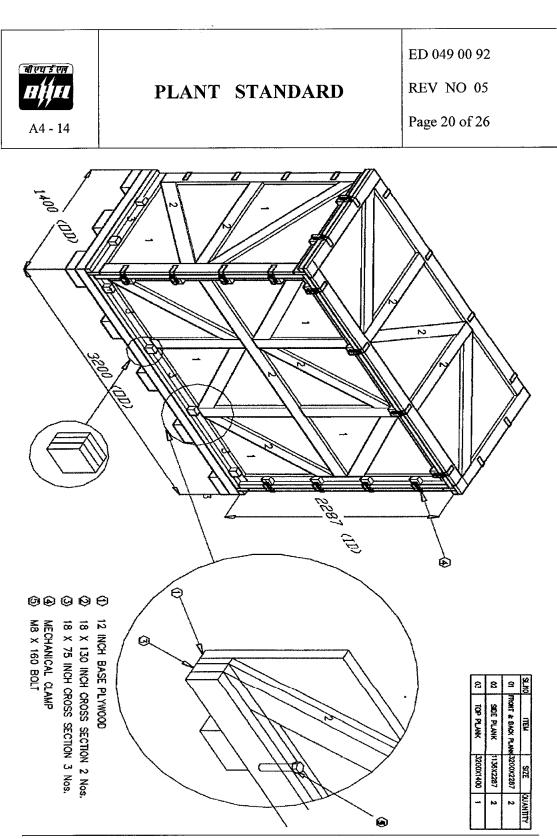
Fig - 8 : CLW Railway Panel Packing with Plywood & Plywood Support Battens
