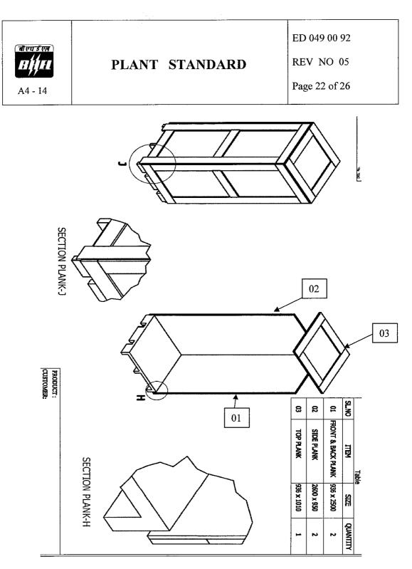
Fig-10 : Plywood Packing for Single Suit Panel.
