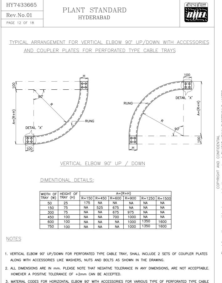
4. THE DETAILS SHOWN IN THE DRAWING ARE TYPICAL FOR PERFORATED TYPE CABLE TRAYS.
