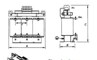
Dimensions in mm A= 450; B=235; C=440; D=316; E=173 F=140; G=22 Mounting hole =  $\Phi$ 12x18 Output connecting bolt size on bus bar - M6 PE terminal bolt size - M8
