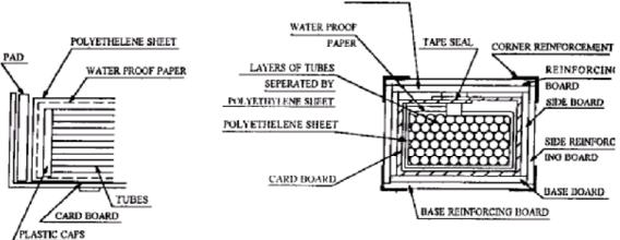
FIG. 1 TYPICAL PACKING OF HEAT EXCHANGER TUBES
