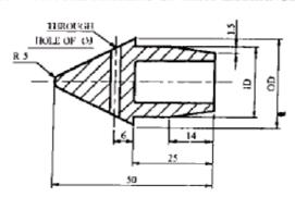
FIG. 2 TYPICAL DRAWING OF CAP FOR TUBE END
