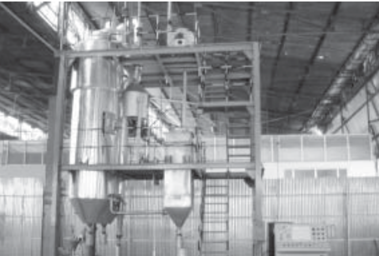
BHEL commissioned Gas-fired Spray Pyrolysis System for pilot-scale synthesis of tailor-made nano materials at CTI Bangalore
