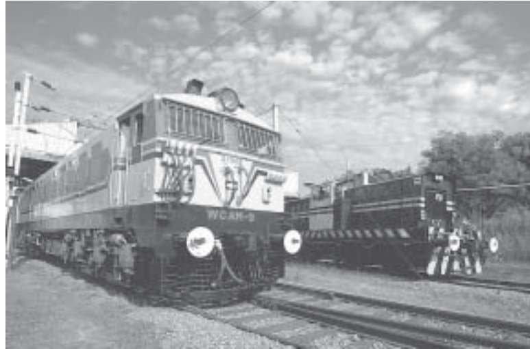
Dual voltage 5000 hp, 25 kV AC electric locomotive
